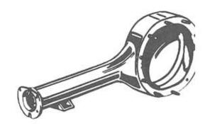
The pre-assembled ABS Power Brake bracket is place on the axle end in place of the original drum brake backing plate. The machined indentation should face out from the axle tube. This is where the original bearing retainer plate will go. The arms that are bolted to the bracket are where the caliper will mount. These arms should face to the back, the caliper will mount to the back of the axle houseing.
